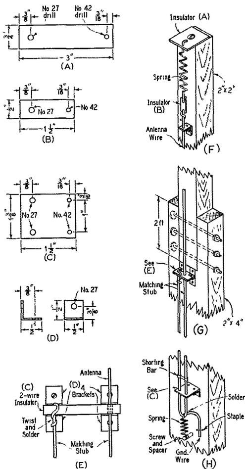
Fig. 2 Detailed sketches of parts and assembly of the simple "J" antenna. A — Top antenna anchorage, 1 required. B — Single-wire insulator, 6 required. C — Two-wire insulator for matching section, 5 required. D — Metal angle pieces for fastening insulators to mast, 17 required. E — Method of mounting two-wire insulator at top of matching section. Four angles are used here. F — Antenna insulator and spring assembly at top of mast. G and H — Details of mast and antenna assembly.
