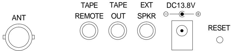
ANT -- connect optional antenna with BNC connector.
