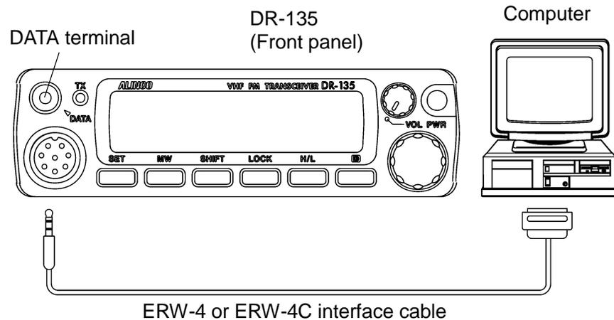
2. Start the Channel Data Editor on your computer. On the main menu, press the **F3** key, and select the “Radio Option (R)” option. In the “Edit option data” window, select the “Channel” option in the “Indication Mode” field. Write your changes in the transceiver memory. The transceiver will then enter the Channel Indication mode. For more information about using the software, see chapter 3 “DR-135 Channel Data Editor”.
