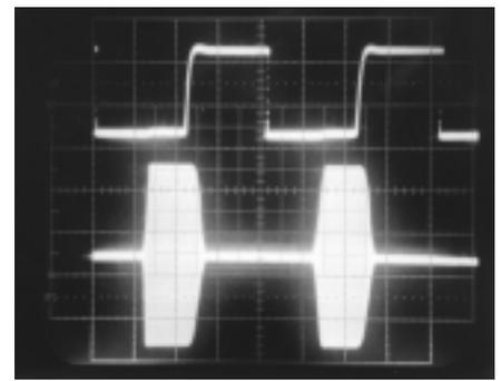
**Figure 3—CW keying waveform for the IC-756PRO showing the first two dits in full-break-in (QSK) mode. The equivalent keying speed is 60 WPM. The upper trace is the actual key closure; the lower trace is the RF envelope. Horizontal divisions are 10 ms. The transmitter was being operated at 100 W output at 14.2 MHz. Note that both dits are somewhat shortened. Only the first dit is shortened in semi-break-in mode.**
