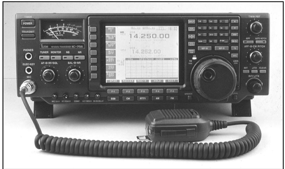
10 memo pads; and four types of scanning. The IC-756 lets you view the contents of nine memory channels at a time (or scroll through them all) via its memory channel screen.
