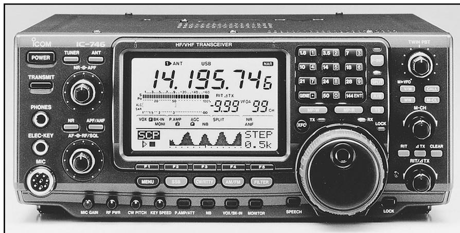
Funmobile stopped by HQ back in June, we got a chance to see both radios side by side. The most noticeable difference is the separate analog meter on the '756. The '746 metering is all on the LCD display. One scale shows signal strength or power output, and two additional meter sections indicate ALC and SWR levels.
