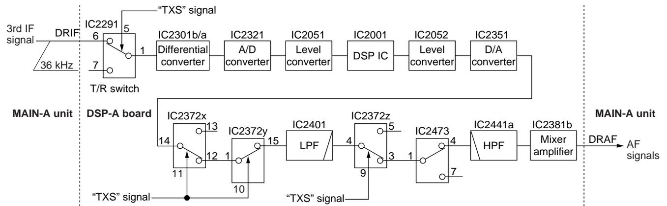
The level shifted signal is applied to the DSP IC (IC2001) for 36 kHz digital IF filter, demodulation, automatic notch and noise reduction, etc. The output signal is level shifted 3.3 V to 5V at the level converter (IC2052), and is applied to the D/A converter (IC2351) to convert into the analog audio signals.
