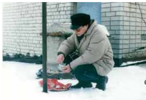
Photo: Finding of resonance of the mast with help a GDO
