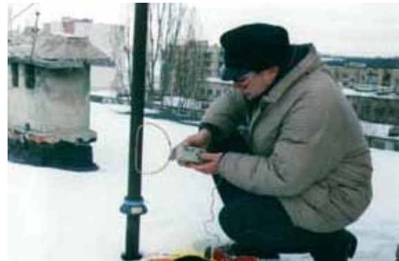
Photo: Finding of resonance of the antenna mast with the ferrite core at its base with help a GDO
