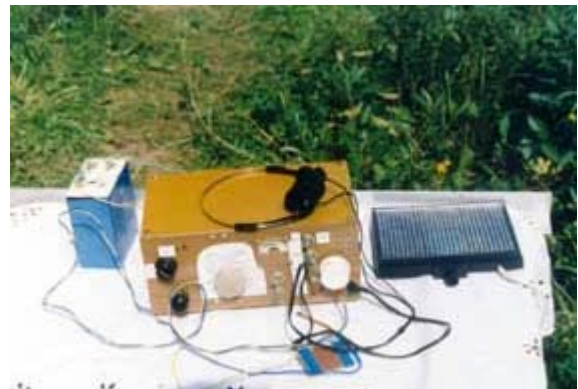
Photo: My QRP transceiver with a Solar battery and such simple key
