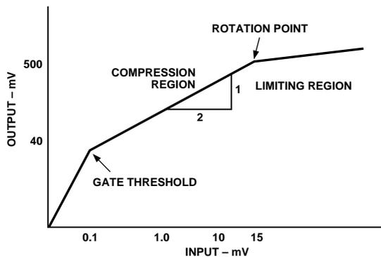
Figure 25. Transfer Characteristic
