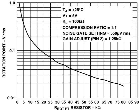
Figure 9. Rotation Point vs. R<sub>ROT PT</sub> (Pin 11 to V<sub>+</sub>)
