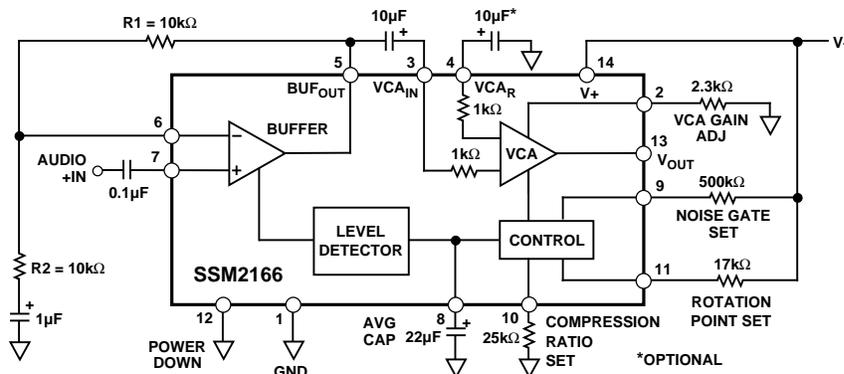
Figure 2. Functional Block Diagram and Typical Speech Application
