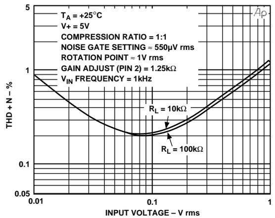
Figure 7. THD+N (%) vs. Input (V rms)
