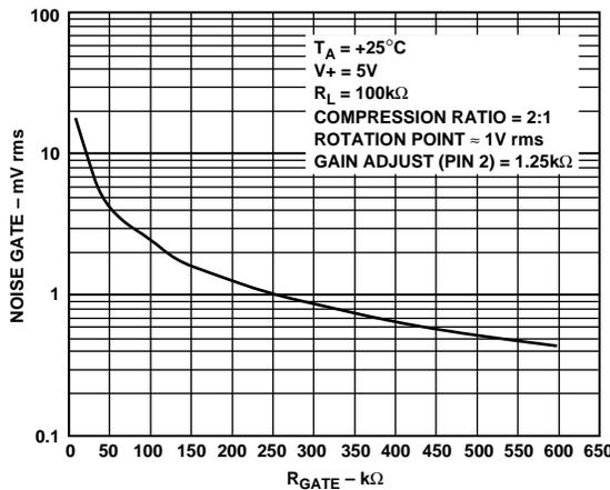
Figure 4. Noise Gate vs.  $R_{GATE}$  (Pin 9 to  $V_+$ )
